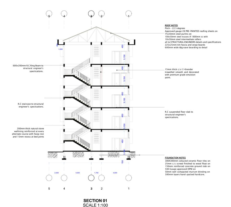
DPM on 50mm thick compacted murrum. 250mm layers compacted hardcore Murrum backfill well compacted in layes of 150mm. 200mm thick masonry wall reinforced at every alternate course. R.C Foundation footing 50mm thick mass concrete blinding.
