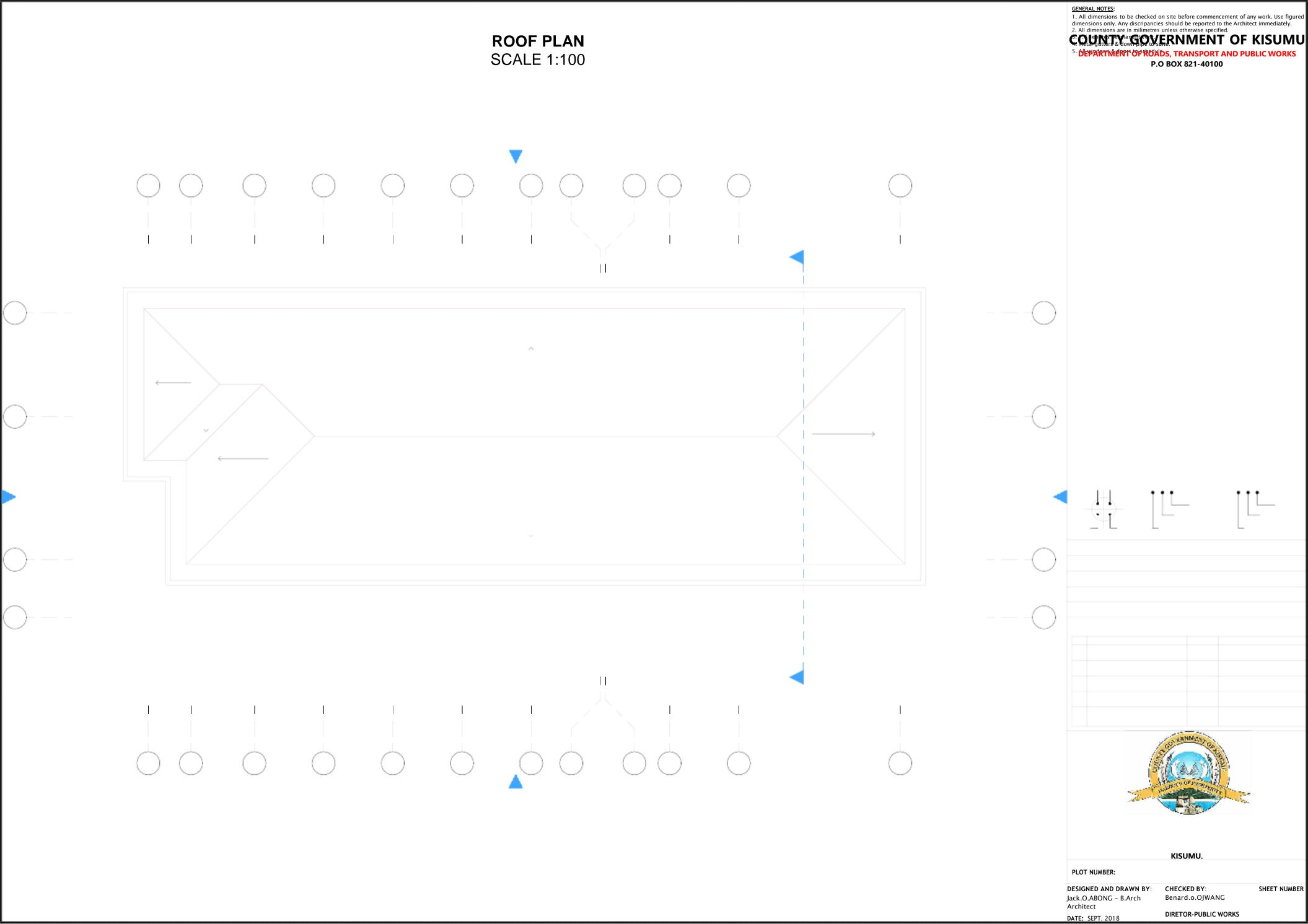
5 4 3 2 ROOF NOTES Pitch – 22.5 degrees Approved gauge 28 PRE-PAINTED roofing sheets on 75x50mm steel purlins on 100x50mm steel trusses @ 1800mm cc with 10x50mm steel intermediate rafters all to STRUCTURAL ENGINEERS details and specifications 225x25mm tim fascia and verge boards 600mm wide t&g eave boarding to detail PRECAST R.C SUNSHADING FIN
