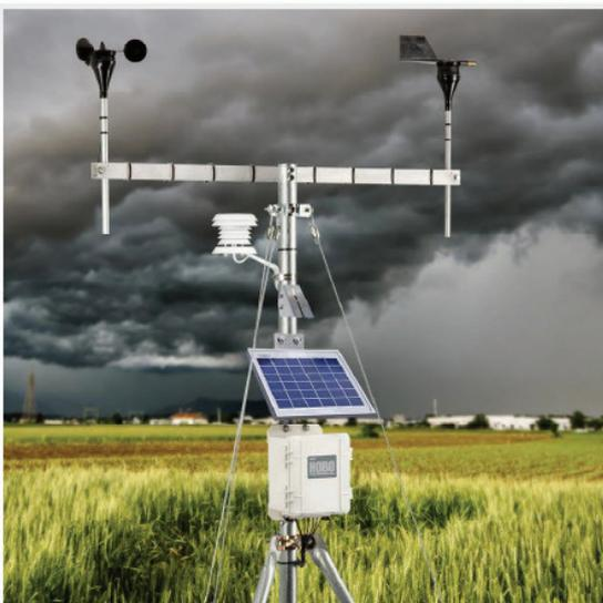
**Consists of remote sensing instruments for measuring; Temperature, Pressure, Humidity, Precipitation, Solar radiation and wind.**
