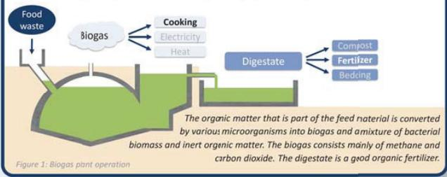
Figure 1: Biogas plant operation
