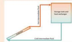
Figure 4: Schematic representation natural convection
