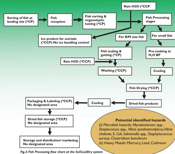
Fig. 2: Fish Processing flow chart at the SolCoolDry system
