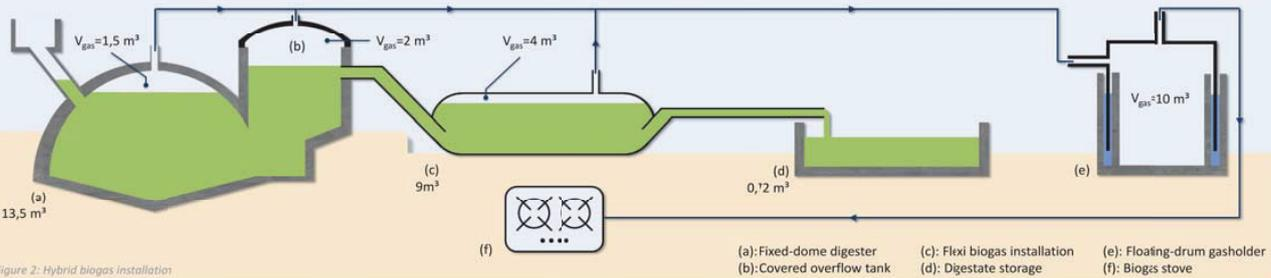
Figure 2: Hybrid biogas installation
